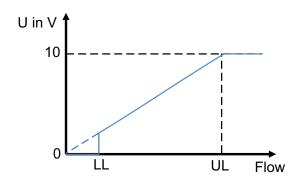
LL: lower limit of measuring range UL: upper limit of measuring range
